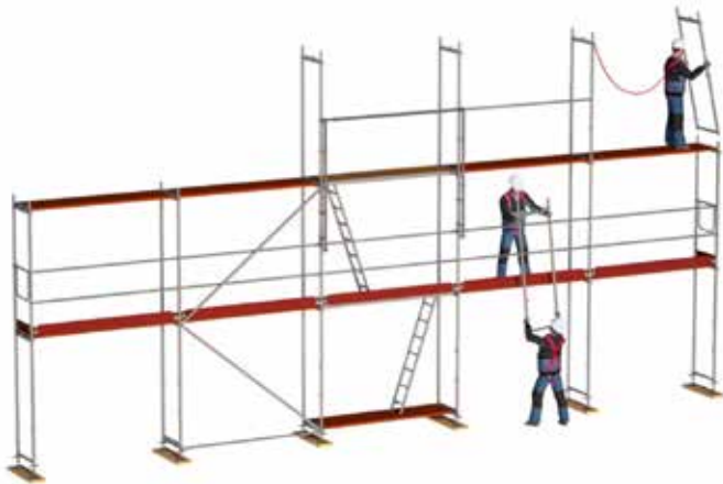
Figure 35: Assembly with personal protective equipment on the topmost scaffolding level
