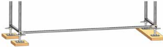
Figure 7: Assembly of the first scaffold bay - longitudinal ledger
