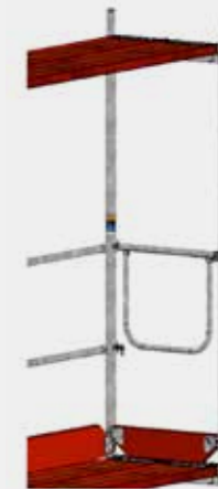
Figure 33: Installed front guardrail: open tube end mounted on a gravity lock
