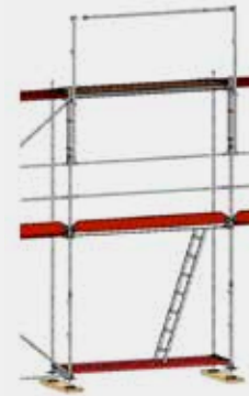
Figure 28: Fitting the second mounting safety guardrail post
