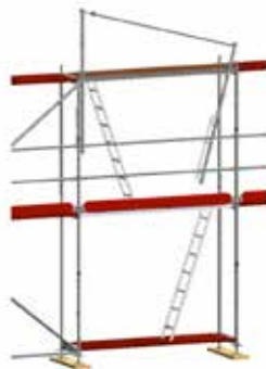
Figure 27: Hooking in the mounting safety guardrail and connecting the second mounting safety guardrail post
