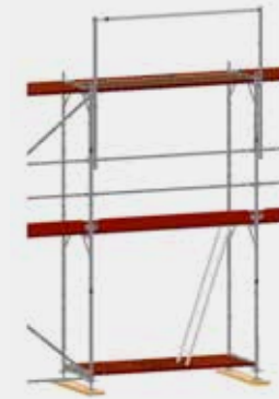
Figure 28: Fitting the second mounting safety guardrail post
