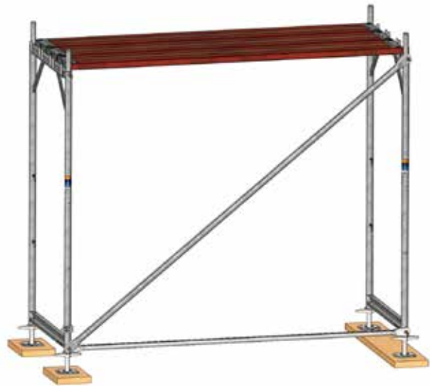
Figure 16: Fully assembled first scaffold bay
