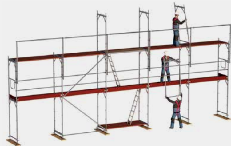
Figure 25: Example of vertical transport by hand
