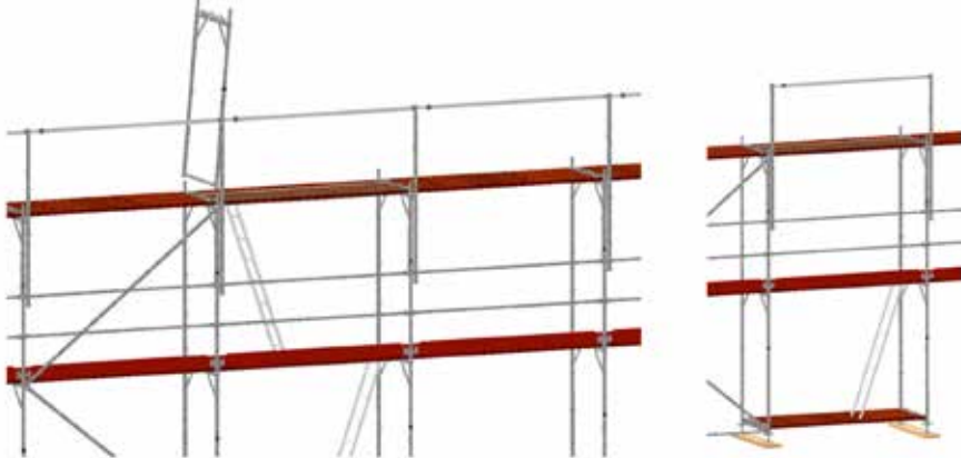
Figure 31: Attaching a vertical frame
